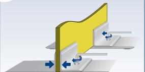
Squeeze the bracket to the panel and tighten the screws.
